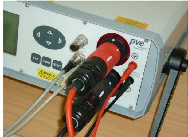
check in practice serves the certainty of the customer and also that of the installer. Beyond that the measured I-V-curves permit further explanations about the electrical characteristics of the verified module or string. So the PVPM is suitable as well as an instrument in research as for development purposes.
