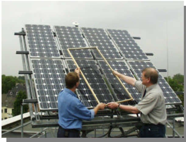
Fig.4. R_s -Measurement of single PV-Modules
